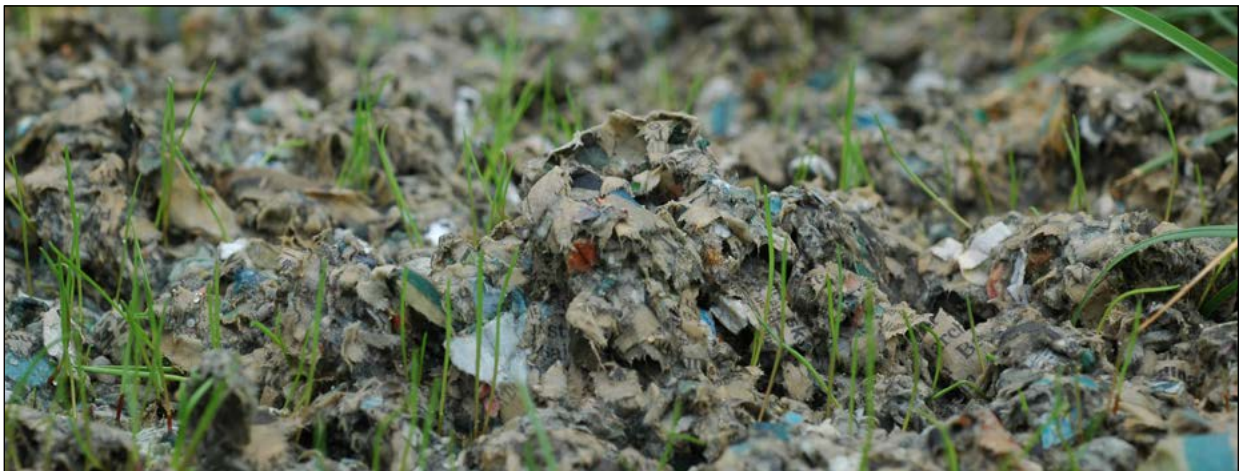
Figure 10. Hydroseeding with grass seed and approximately 1,200 pounds of fiber mulch per acre has been most successful in preventing the blowout of seed and sand.
