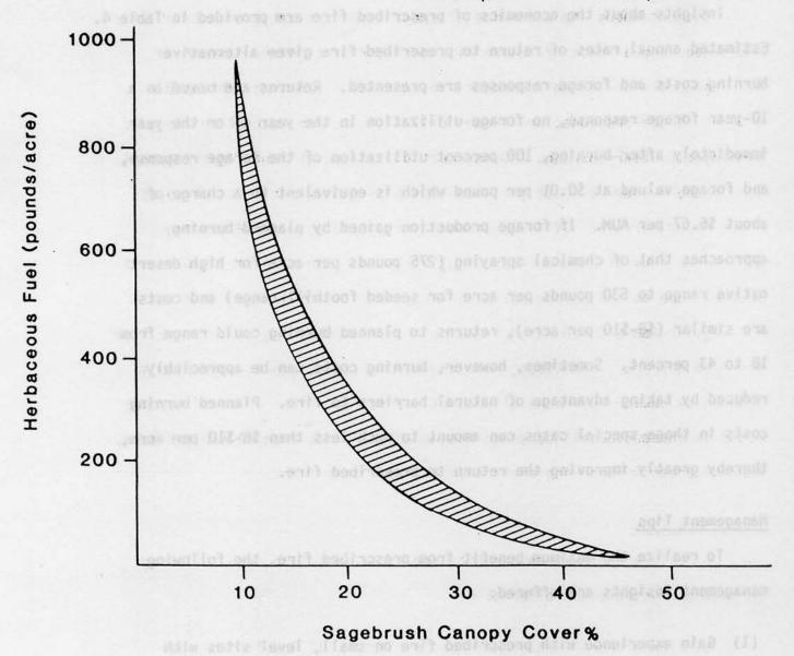
Figure 3. Approximate relationship of sagebrush canopy cover and herbaceous fuel loading for successful fall burning in eastern Oregon.
