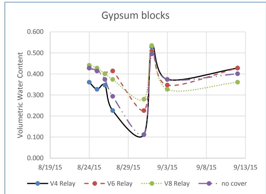
**Figure 3.** Soil moisture measurements from one replication in treatments 1, 2, 3 and 12 from mid-August until harvest with three different monitoring systems.
