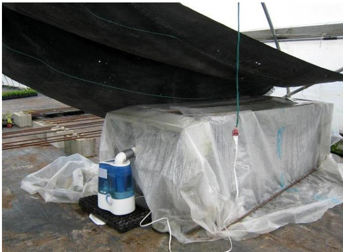
(Figure 4) alternative healing chamber design using PVC framework
